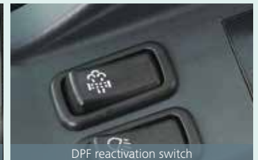
DPF reactivation switch
