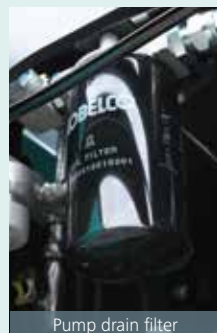
Pump drain filter
