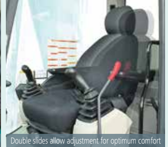
Double slides allow adjustment for optimum comfort
