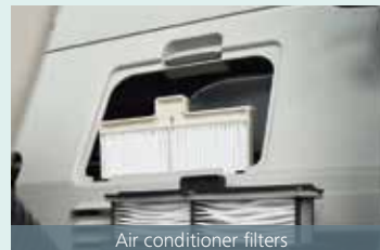
Air conditioner filters
