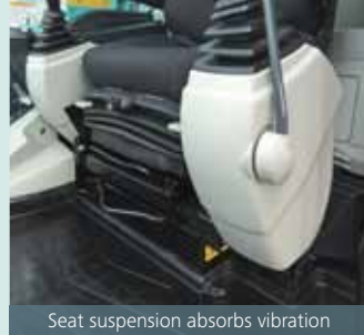
Seat suspension absorbs vibration
