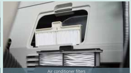
Air conditioner filters
