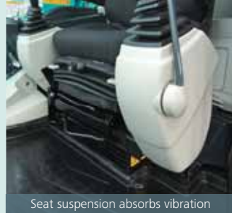
Seat suspension absorbs vibration
