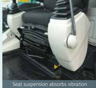
Seat suspension absorbs vibration
