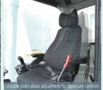
Double slides allow adjustment for optimum comfort
