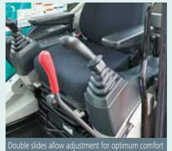
Double slides allow adjustment for optimum comfort
