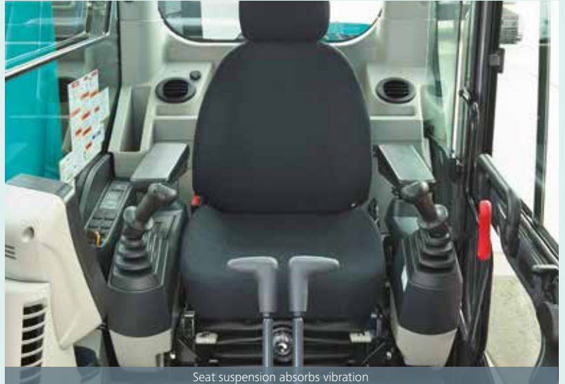
Seat suspension absorbs vibration
