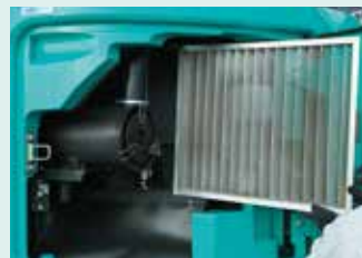
iNDR filter/radiator reservoir tank/air cleaner
