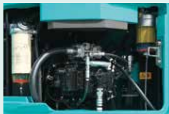
Fuel filter with built-in water-separator
