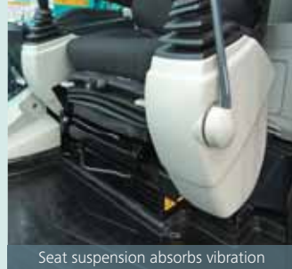
Seat suspension absorbs vibration
