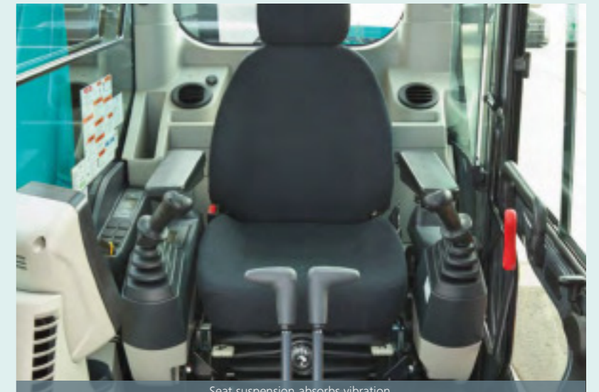
Seat suspension absorbs vibration
