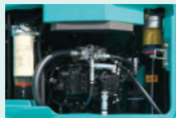
Fuel filter with built-in water-separator
