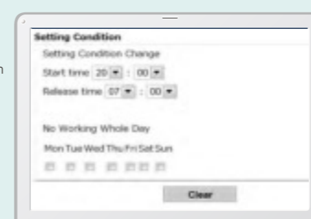
Engine start alarm outside prescribed work time
