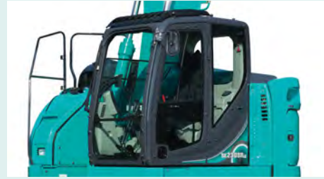
Mounting brackets for vandalism guards are standard equipment (contact your KOBELCO dealer to fit vandalism).
