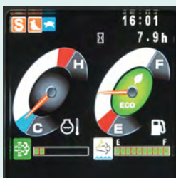
PM accumulation display (left)/ Urea level gauge (right)
