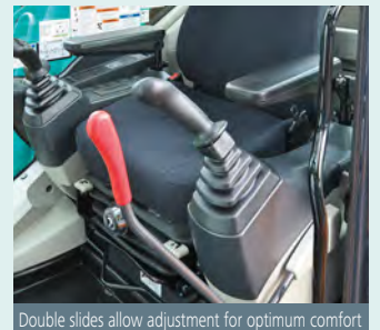
Double slides allow adjustment for optimum comfort
