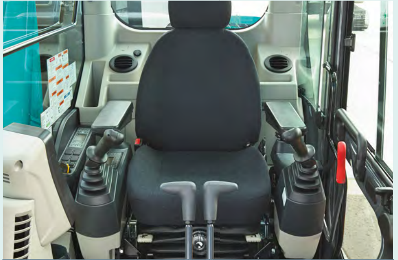
Seat suspension absorbs vibration
