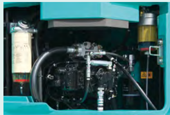
Fuel filter with built-in water-separator
