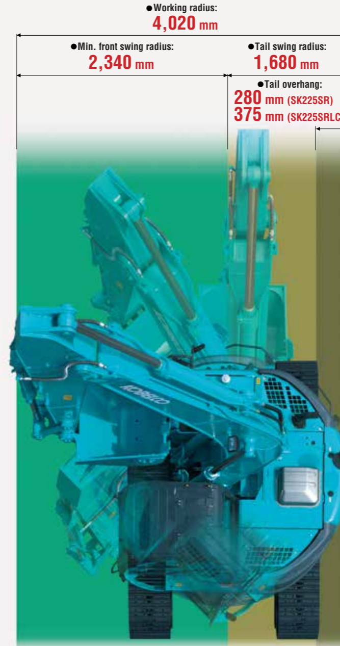
***Working radius** equals the sum of the minimum forward swing radius and tail swing radius.
