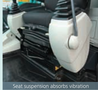
Seat suspension absorbs vibration
