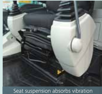
Seat suspension absorbs vibration
