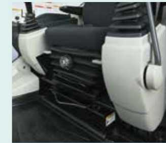
Seat suspension absorbs vibration
