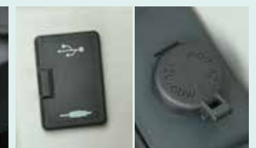
USB connector/12V power outlet
