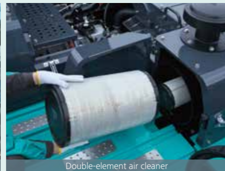
Double-element air cleaner
